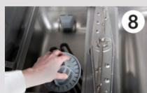
Put back the pump filter turning clockwise to lock position.
