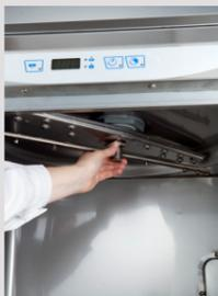
Unscrew the upper rinse arm. Pull the wash arm. Remove both and clean.
