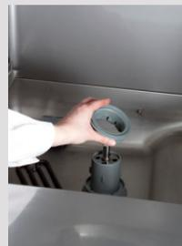
Turn the ring gasket on the centre post counter clockwise to remove. Clean it.
