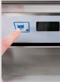
Close the door and **press the drain cycle button once**
