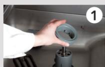
Put back ring gasket turning clockwise to lock position.
