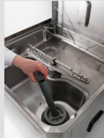
Remove the overflow pipe.
