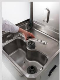
Lift the lower wash arm. Remove and clean.
