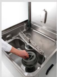
Lift up and remove the wash pump filter.
