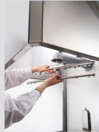
Remove the upper wash arm. This will drop down when you remove the rinse arm. Clean it.
