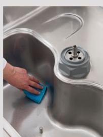
Clean out any residue left in the tank. Wash down all walls and surface areas.
